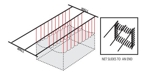
This indoor tunnel ceiling suspension kit is ideal for any gymnasium or other multi-use training facility with a high ceiling. Support cables are hung across side walls and additional vertical cables extend to attach the batting tunnel net. This unique design allows it to be installed at any height customized specifically to your location's needs. When the indoor batting tunnel net is not in use, the net is easily stored by sliding it to one end of the facility and out of the way.
