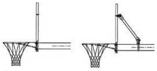
(5) Install board to post using two of the 3/8 x 1" bolts (supplied with the backboard) in the top and bottom holes on the center of the plate. Depending on the type of board being installed, the bolts required will be either a carriage bolt (used with steel boards) or the flat head bolts (used with aluminum boards).
