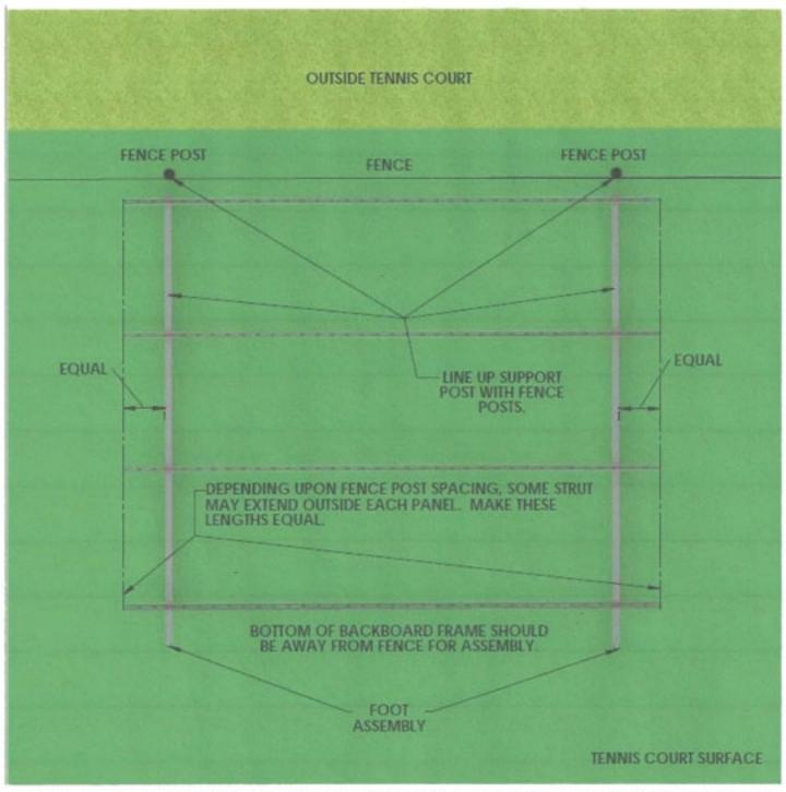
NOTE: THE SUPPORT POST WILL ATTACH TO THE FENCE POSTS. THE STRUTS WILL BOLT TO THE SUPPORT POST AT WIDTHS EQUAL TO THE WIDTH OF THE FENCE POST CENTER-TO-CENTER.
